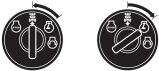
Engine "ON" Position (Normal Operating)
